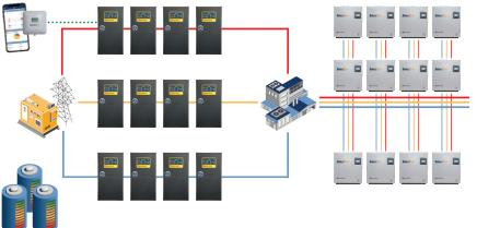
240kW of continuous load power can be achieved, using 4x 20kW SP PRO inverters per phase on a 3 phase system
